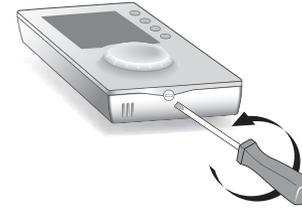
Unscrew the terminal box cover and lift it up as high as it will go to block it, then position the base on the wall running the wires out through the hole in the cover.
