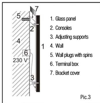
**The panel has to be installed in such a way that the V26 receiver is always in the bottom part of the panel.**
