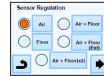
Select the chosen sensor regulation by pressing on the touch button near the sensor regulation possibilities. The active touch is colored red. Press the ▶ key in the bottom right corner to continue to the next part of the installation. You can return to the previous menu by pressing the ↶ key.
