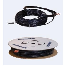
**PSV heating cable** – a single-conductor cable with a full protection screen for storage and semi-storage heating. Cold lead 2×5 m. 230 V. Cable diameter 4.5–4.8 mm.
