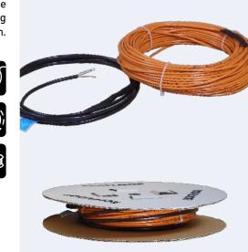
▶ ADPSV heating cable – a twin conductor cable with a full protection screen suitable for semi-storage and storage floor heating in living areas. Class M2. 1×5m cold lead. Ø 5.3–5.9mm. 230 V.
