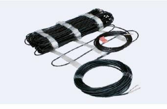
► ADSV+ heating cable – a two-conductor cable with a full protection screen. The sheathing of the cable is resistant against UV radiation and is intended for floor heating and the removal of snow and ice from roofs and eaves troughs. 1×3 m cold lead. Ø 5.0 mm. 230 V.
