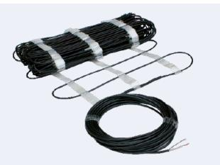
ADPSV heating cable / mat – a twin conductor, full protection screened cable with protection against UV radiation. This multipurpose cable is suitable for indoor and outdoor applications. Class M2. 1×5 m cold lead.  $\varnothing$  5.0–5.9 mm. ADPSV heating mat: width 0.5 m. Packed in PE foil.
