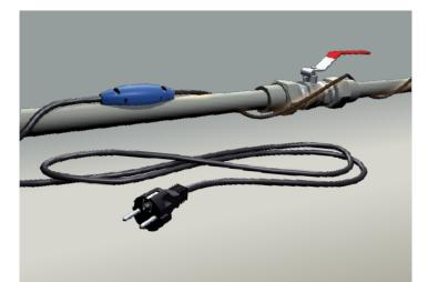
▶ MAPSV heating cable – a single-conductor cable with a full protection screen and protection against UV radiation. Suitable for heating outdoor surfaces. Cold lead 2×5 m. Ø 5.9–6.4 mm. Packed in PE foil.
