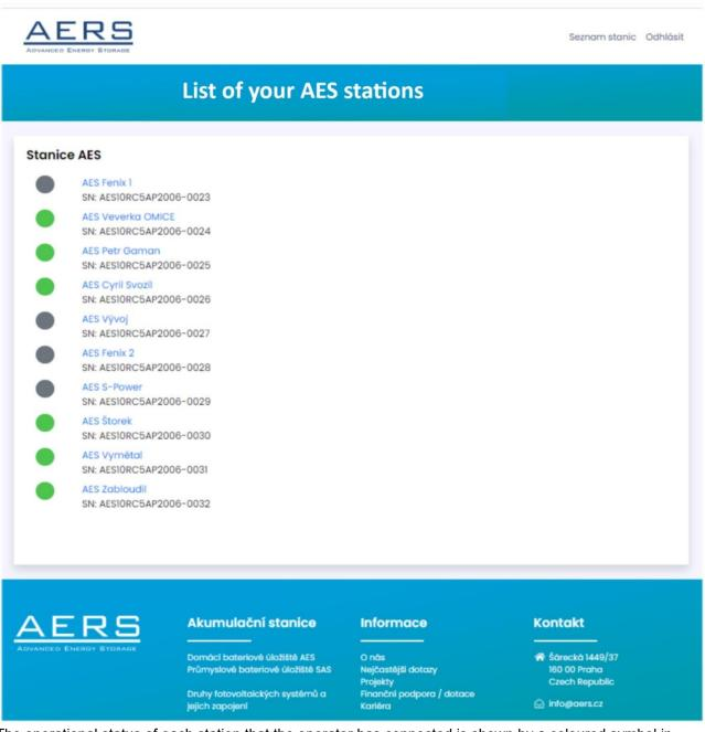
The operational status of each station that the operator has connected is shown by a coloured symbol in front of the project name.
