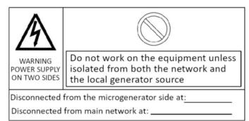
The HES6/10 station is equipped for mounting connection terminals on both the right and left side. Access to the terminal block is covered by a side plate. The position on which side the terminal block is located is marked on the respective side part with the following label according to EN 50438ed1.
