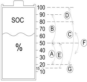
(A) – Range of 20 to 50% SOC. This range is intended for the capacity reserve of the station operation in island operation or in the operation of controlled compensation of grid consumption in times without solar energy (reduction of the power drawn from the grid, at high coincidence).
