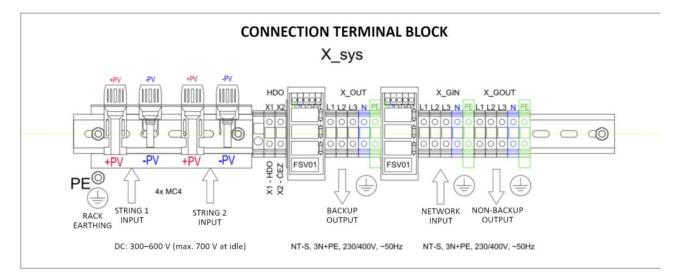
**The means for disconnecting the DC** leads are implemented on the X\_sys connection terminal block. This terminal block serves as a single point for the connection of the supply and output cable and the connection of the equipment to the internal installation of the building.
