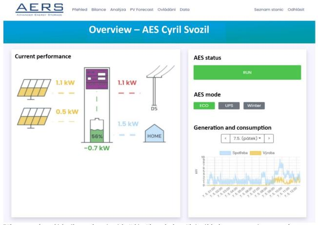
When entering the control interface, each user has an immediate view of the operational status of the station, which is shown on the "Overview" page. On this page, the instantaneous values of the operating variables in minute average are shown in individual blocks. A negative sign on the power display for batteries indicates charging at the indicated power.
