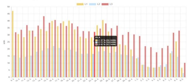
The difference of values in the individual graphs "Consumption by phases" and "Distribution consumption by phases" represents the energy delivered to each phase from its own generation.
