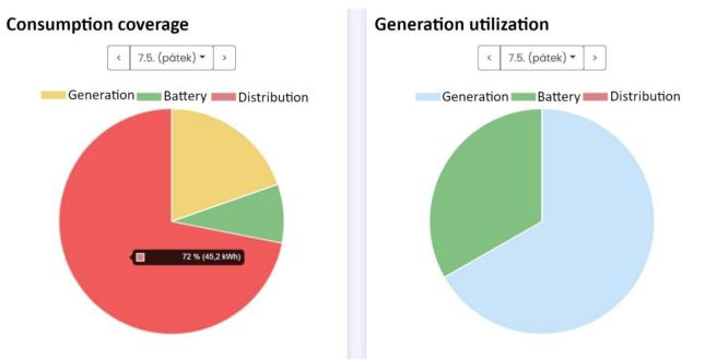
The "**Consumption coverage**" diagram shows how much the different sources, i.e. the distribution network, the solar panel generation and the energy stored in the batteries, contributed to the consumption of the building. The user has access to the exact values of the averages by placing the cursor on a specific area of the diagram.
