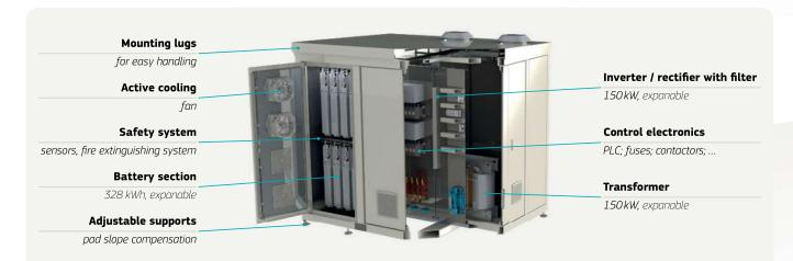
**Battery section /** We use battery modules previously used in ŠKODA electric cars. In each of the two sections there are 24 series-connected modules in a suspended system that allows quick replacement and ensures optimal circulation of cooling air. The battery sections are constantly monitored. Each section can be shut down separately, and so some of the batteries can be replaced without the need for a total shutdown.
