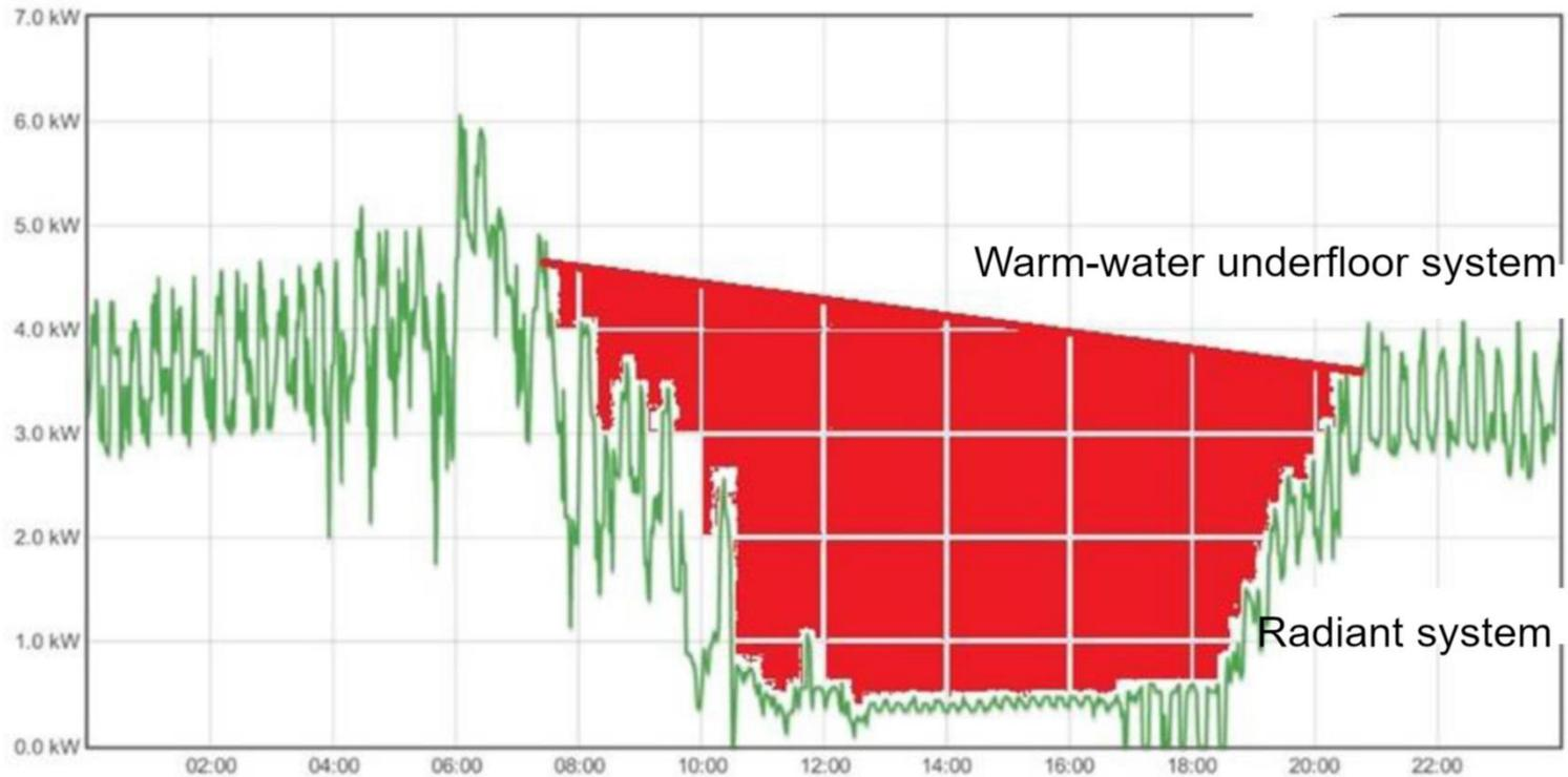
This graph depicting the energy consumed by heating shows the significant influence of heat gains (sun - people - technology) on the building's energy consumption. In order to exploit this effect fully, it is essential to use a flexible heating system capable of reacting swiftly in each individual heated area.
