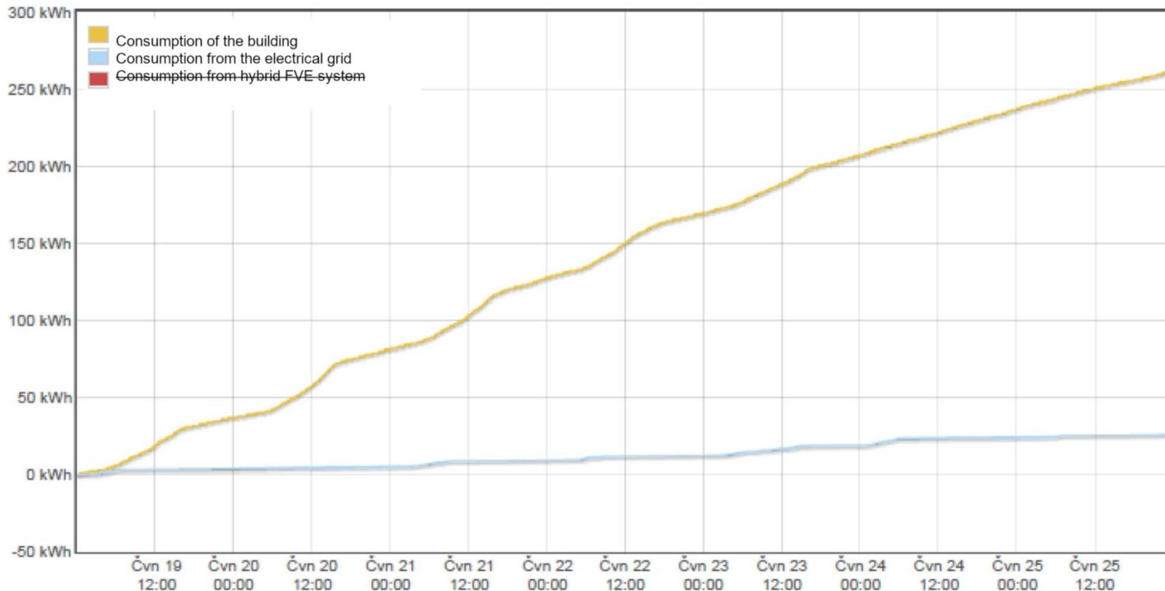
**The output of the PVS covered 91% of the energy requirements of the building under these conditions.**
