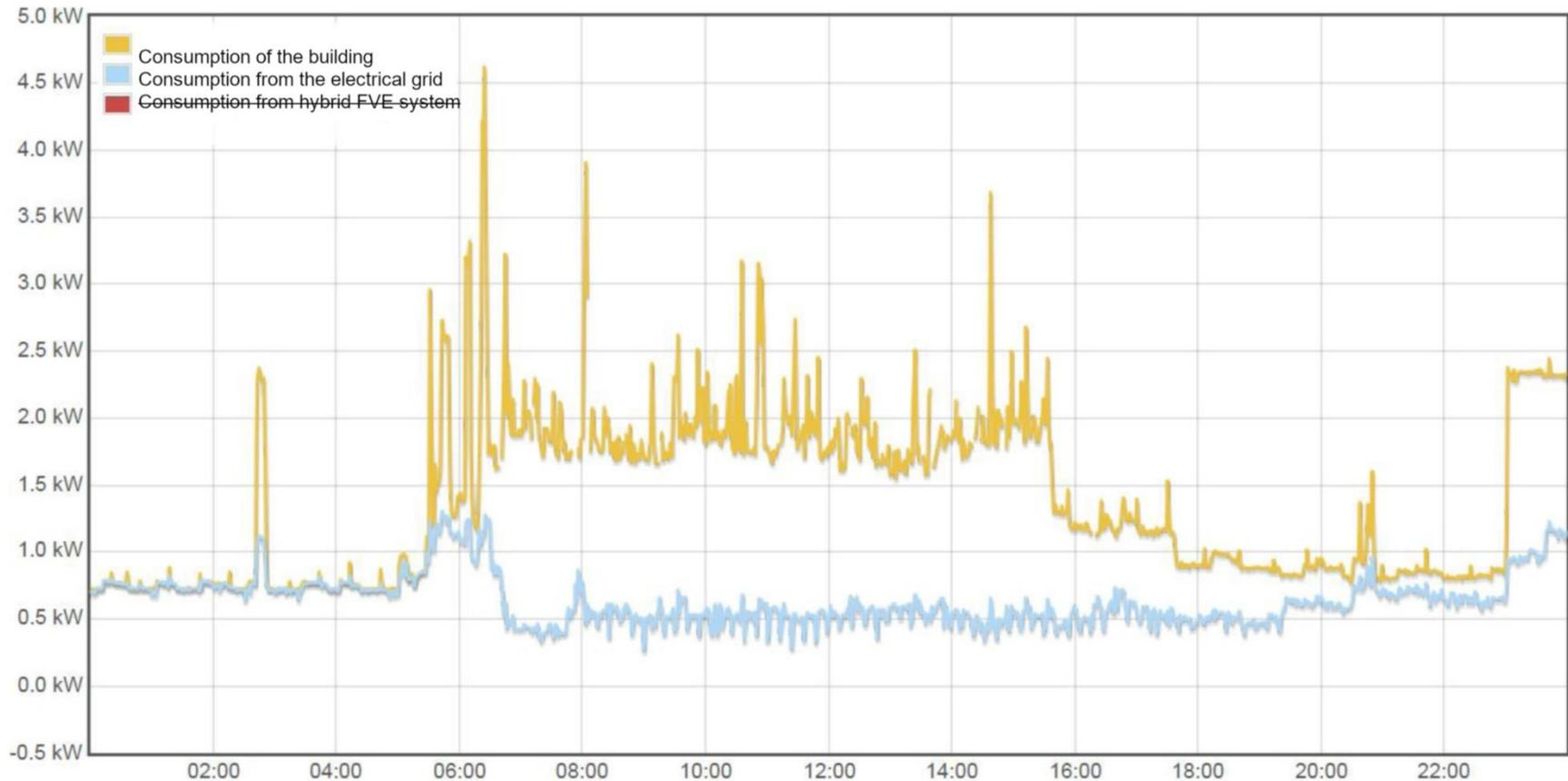
The maximum total electricity consumption of the building was 4.5 kW
