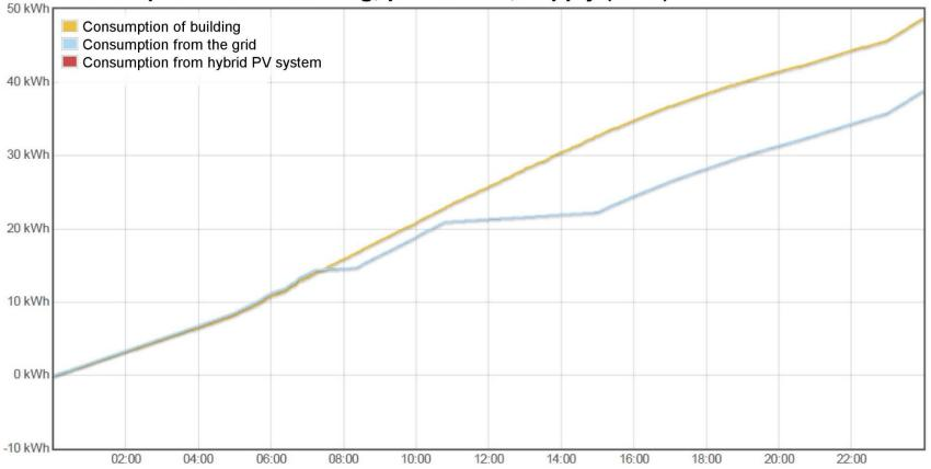
Total consumption of the building was 48 kWh, supply from the network – 35 kWh
