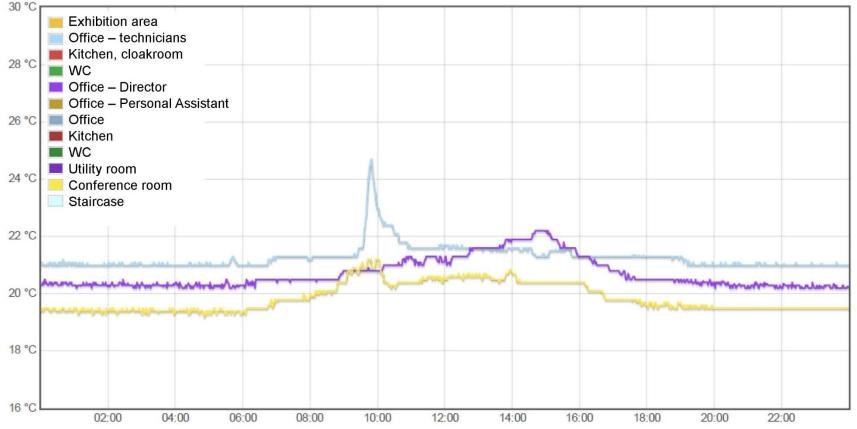
The visible sharp increase in temperature around 10 a.m. and 3 p.m. is caused by the direct exposure of sensors to sunlight (the outdoor blinds are not operational in the winter due to the use of heat gains from sunlight). This phenomenon has now been prevented via the installation of indoor scattering blinds.
