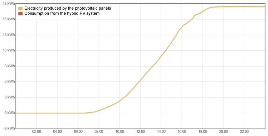
The PV system produced 17 kWh on its own, 100% of which was used in the building.
