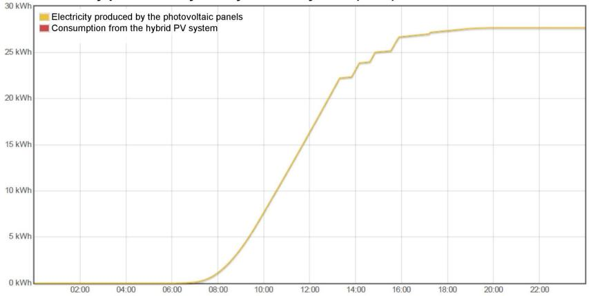
The PV system produced 26 kWh of electricity, of which 100% was used in the building!
