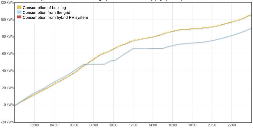
The total energy consumption was 102 kWh, while the PV system covered 21 kWh, i.e. almost 21% of the energy requirements of the building!
