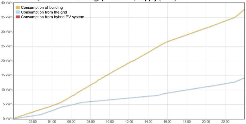
The real energy consumption in the building was 38 kWh, during which only 12 kWh was drawn from the grid.
