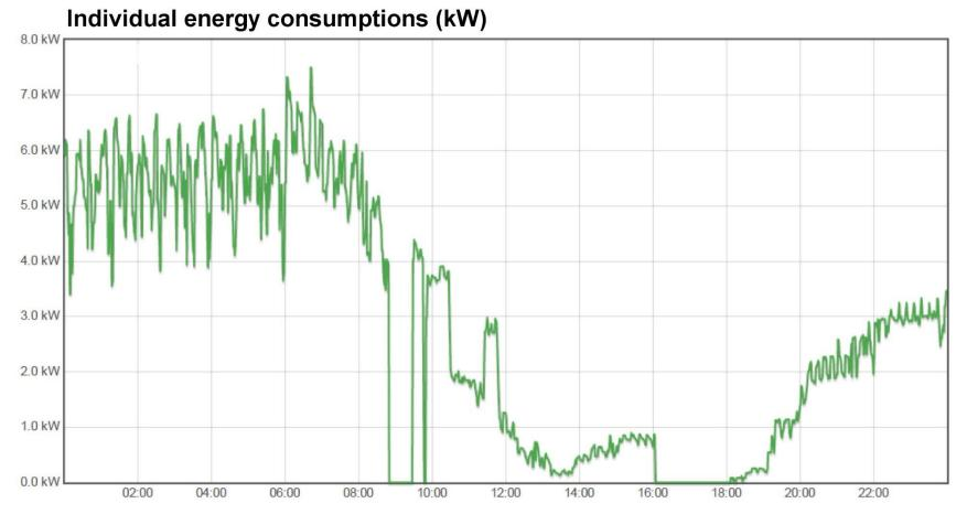
The significant effect of heat gains (sun-people-equipment) on the energy consumption can be seen from this graph, which shows energy consumption for heating. In order to make full use of this effect, It is essential to use a flexible heating system capable of reacting swiftly for each heated area independently.
