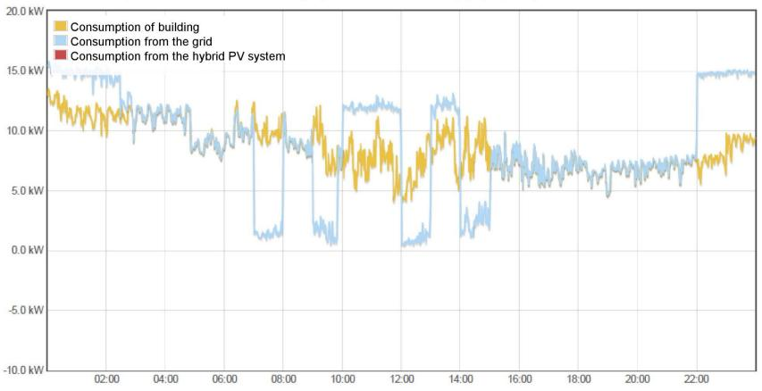
It is clear from the graph that with regard to the technical parameters of the building, the consumption of energy over the 24 hour cycle is very even (the main consumption is from the radiant heating). Even under these conditions, this concept ensures controlled zero consumption by the building from the grid for a period of 4 hours.
