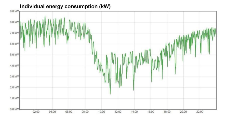
Energy consumed for heating (by the radiant heating system) reacts flexibly to the change in outdoor temperatures and particularly to additional heat gains (people – equipment)
